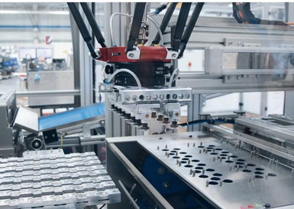
Top: Transition from the Blister Machine KBS-PL to the Blister Machine KBS-KF
