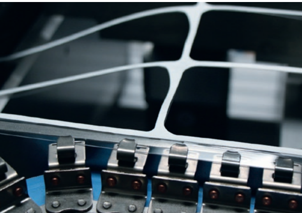
Above: With the KBS-KF blister machine, the clever placement of the blisters after die-cutting leaves only a little material remains.
